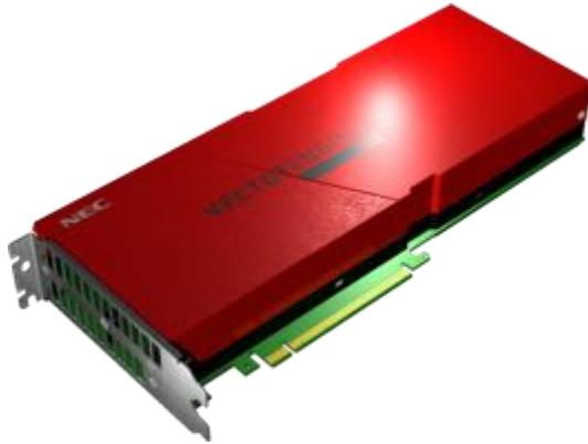
There are eight vector core in each processor. This might seem few to those unfamiliar with vectors processors. Let's just say that each core is able to perform up to 192 double-precision floating-point operations per cycle. With a 1.6 GHz clock frequency, this lead to a 307.2 GFLOPS per core for a total of up to 2.45 TFLOPS per chip.
